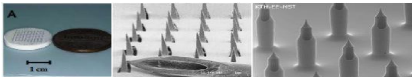
Figure 8: (from left to right) Dissolving microneedle array 41 ; Solid microneedle array with hypodermic needle for comparison 42 ; Hollow microneedle array 43
